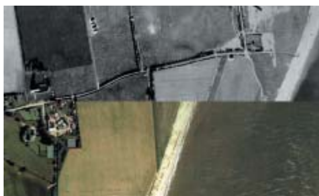
Left: Erosion of over 250m of the Suffolk coastline, UK between 1940 and 1999. © RAF and Getmapping plc
