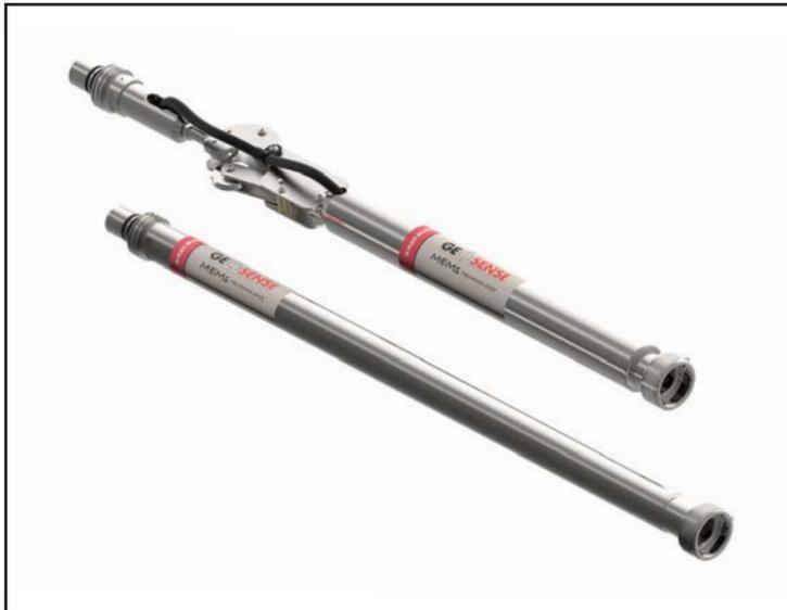
The GXM-A Plus is an Automatic Magnetic Extensometer combined with an In-Place Incliner which can be used typically to measure vertical and horizontal displacement in embankments, dam foundations, deep foundations and around tunnels and diaphragm walls.
