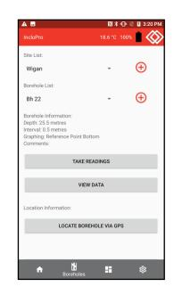
Since any sensing system can be affected by temperature gradients over its electronics and their mountings, the Geosense<sup>®</sup> App automatically monitors the temperature inside the probe. If temperature changes are deemed to risk affecting the data the App will display 'Probe Temperature Stabilising' and will display the current temperature.
