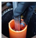
**STEP 16** - Carefully lower the probe into the access tube until it reaches the base of the tube, or the required depth.
