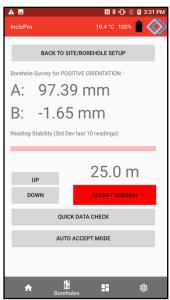
calculates the standard deviation across those readings to measure the difference. It is recommended to wait until the stability bar (and 'Accept Reading' button) shows green before accepting a reading, but this might not be possible if there are external vibrations near the borehole.
