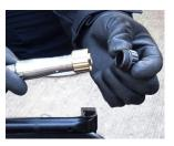
**STEP 3** - Taking note of the machined mating 'D' alignment in the plug and socket and the alignment markers, carefully connect the cable to the probe. Place the probe in a position where it can't fall or be damaged.
