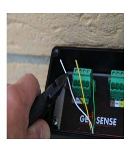
16. Using a small flat screwdriver, connect the conductors into the terminal on the circuit board. The number and colours of the conductors and the connectors used will depend upon the type of output selected.
