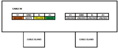
NOTE: IF AN END OF LINE TERMINATION RESISTOR IS REQUIERED THEN THIS SHOULD BE TERMINATED BETWEEN [A+] & [B-] ON THE UNUSED LINE END CONNECTION
