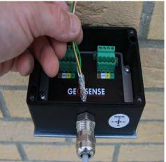
Trim out any 'fillers'. (These are solid plastic cores used to fill the voids in the cable. They have no conductors within them and are white in colour.)
