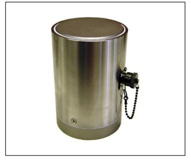
The Geosense® SGLC 7050 series load cell consists of a solid cylinder of high strength stainless steel with a series of electrical resistance strain gauges connected around the periphery as a Wheatstone Bridge that compensates for unevenly distributed loads and provides a single mV/V signal output.
