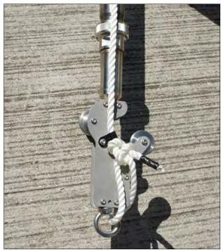
**STEP 8 -** Connect the first extension rod to the bottom wheel assembly making sure to check the 'pin - socket' alignment and tighten the connector until the locking clip 'snaps' into place.
