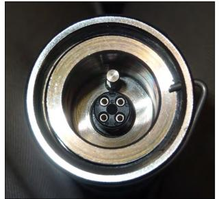
**STEP 4 -** Offer the male connection on the bottom wheel assembly to the female connection on the bottom sensor aligning the positions of the locating pin and socket.
