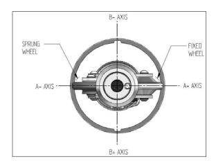
The A axis is the primary axis and the B axis is the secondary axis. Uni-axial IPI sensors only detect changes in the A axis.
