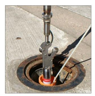
**STEP 22** - Loosen the safety rope and lower the assemblies into the inclinometer casing ensuring that the wheels are aligned in the correct grooves
