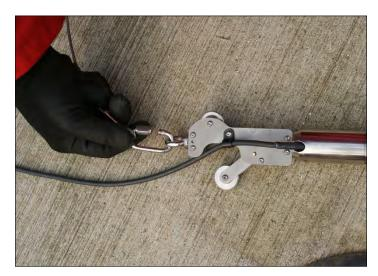
**STEP 18 -** attach the other end of the top support wire to the top collar hanger
