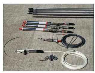
**STEP 2 -** Remove the **BLACK** end cap from the end of one of the rods.
