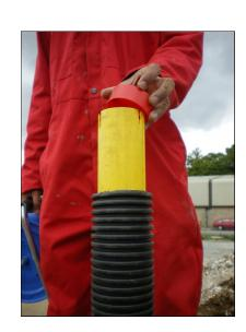
4. Once the probe has reached the bottom of the access tube slowly raise it.
