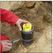
24. Attach the next access tube length to the installed access tube.
