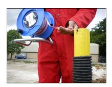
5. Raise probe to next magnetic target and repeat the above reading process. Repeat for all targets.
