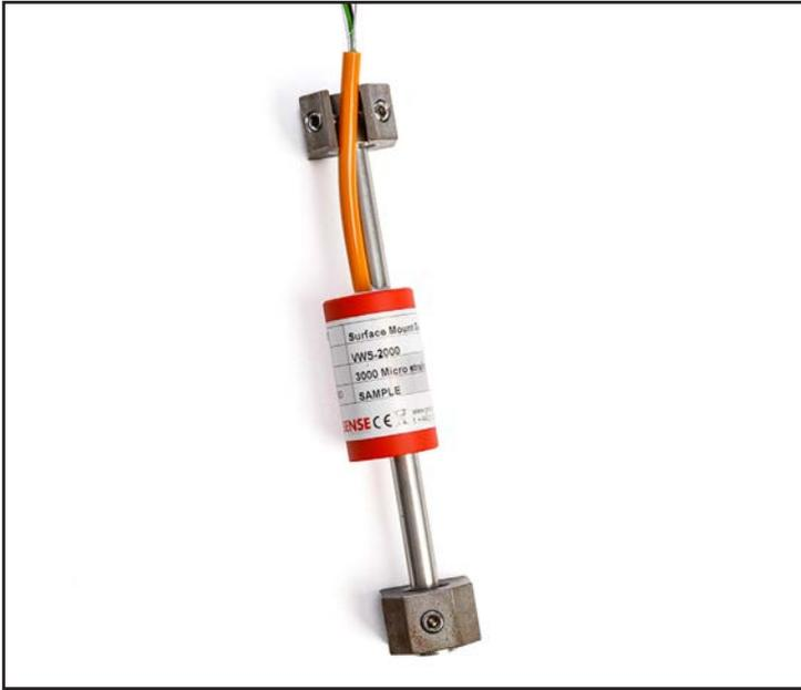
Geosense® VWS-2000 series vibrating wire surface strain mount gauges are designed for the long term monitoring of steel or concrete structures. Gauges may be attached to steel structures by arc welding or, using alternative end blocks, bonded or grouted into concrete.
