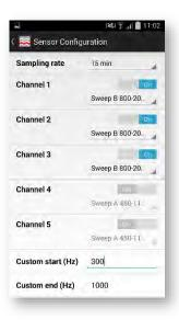
**NOTE**: by default, a new datalogger has all channels set as "Off" for battery saving. Turn to "On" all channels used in order to get data from the sensors.
