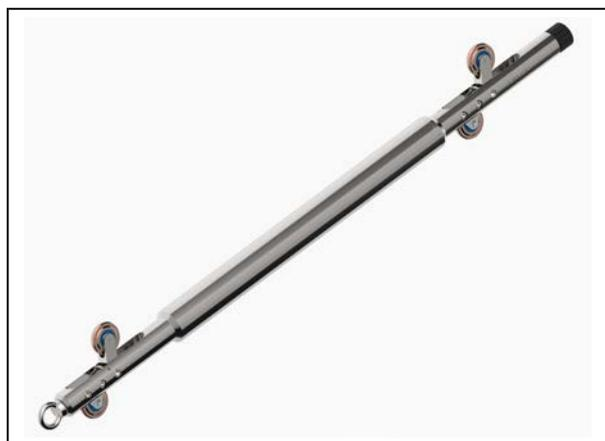
The Geosense Inclined Portable Inclinometer system is used to measure lateral movements and deformations of soil, rock and retaining structures within or on an inclined borehole or surface. Typical applications include monitoring the downstream face of concrete faced rock-filled dams.
